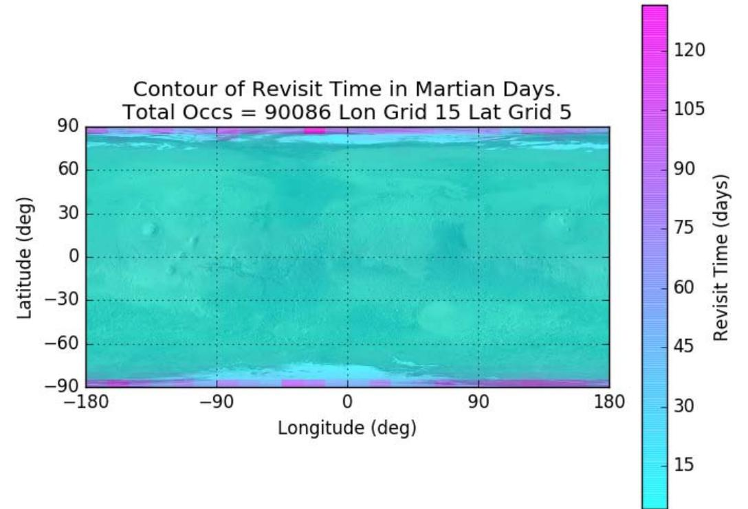
Simulation results of a four satellite constellation at 92 degrees of inclination at altitudes **330, 706, 1350, 3098 km** show **global coverage** for a grid of 15 degrees in Longitude and 5 degrees in Latitude
