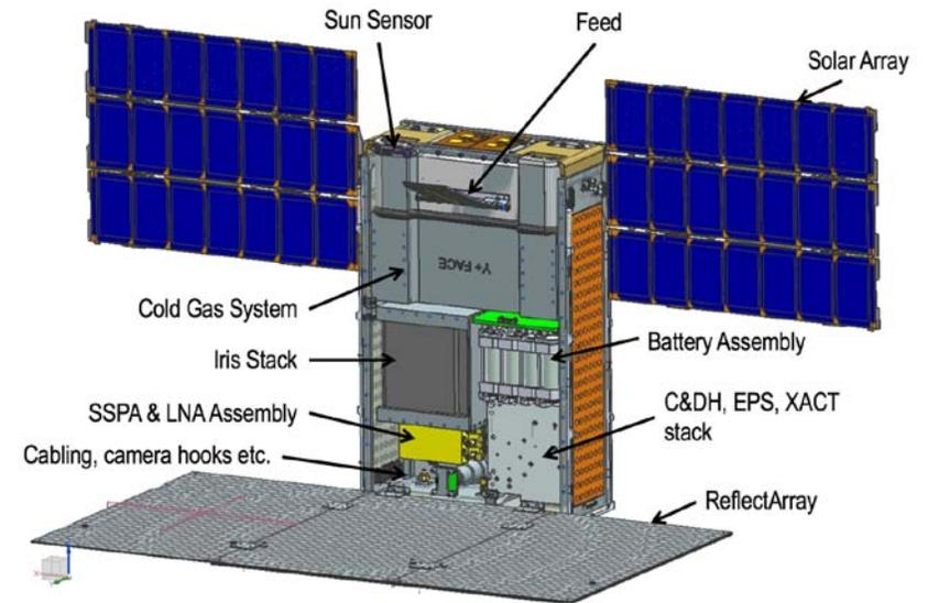
The IRIS fits within 6U cubesat designs such as the JPL developed MarCO cubesat.
