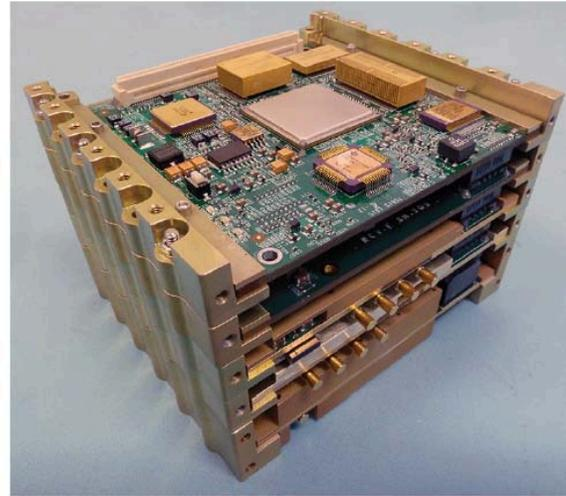
The instrument can be built around the standard IRIS radio. The radio provides transmit and receive capability, operates at UHF, S, X, and Ka bands, and includes data processing capability.
